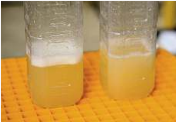
JADAM wetting agent water test. Mix a few drops of JWA, the water should remain clear. Shake, then there should be lots of foam
