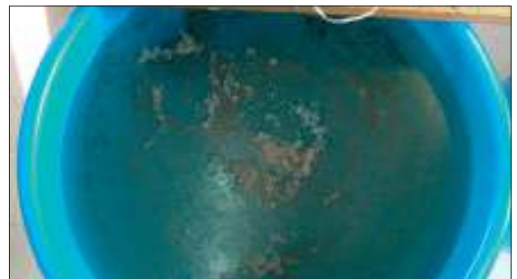
16. All foam has disappeared, leaving behind a film. Microbes have perished. This is not suitable as JMS, but good for liquid fertilizer. (144 hrs)
