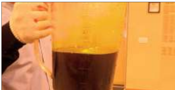
46. This is JS with sediments after taking out 80 L (21.1 gal) of clear JS.
