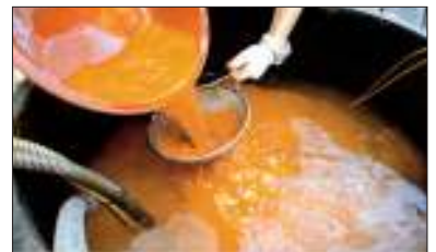
3. Filter out large particles.
