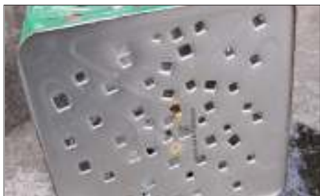
4. Make slightly larger holes on the bottom.
