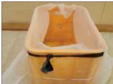
3. Fix the net tight on the box with a thick rubber.
