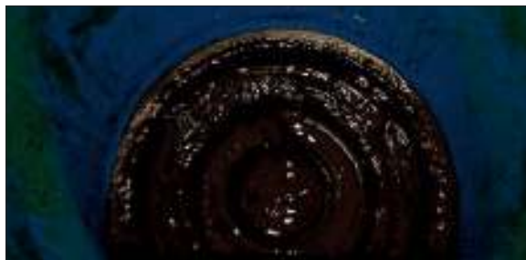
49. What remain at the bottom of the container are phyllite and red clay powders that have not melted completely.
