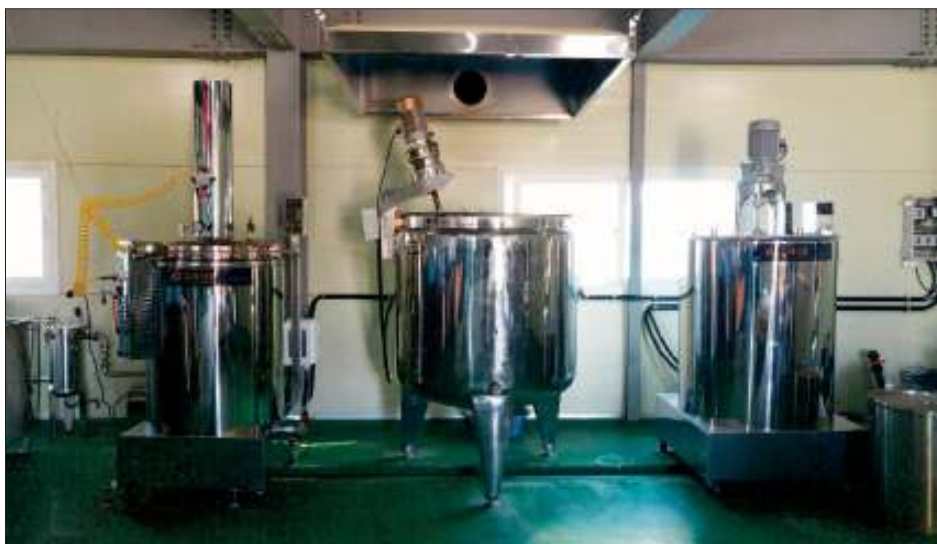
Machines used in Bongha village (CEO Jeongho Gim), Korea, where 160 households came together to farm in JADAM method over 132 ha (330 acres). They produce JADAM pesticide in large scale using these machines. Left is high-pressure pot for boiling herbs. Center is for making JADAM sulfur. Right is JADAM wetting agent. JADAM method can be easily practiced for areas over hundreds of hectares/acres.
