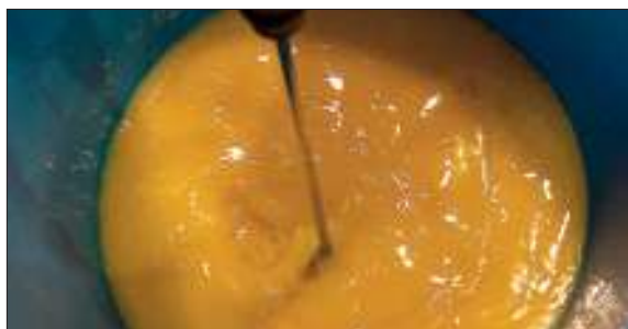
14. Color keeps changing and viscosity increases. 4 minutes passed.
