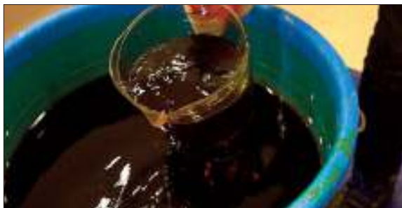
42. Take out the upper portion being careful not to agitate the sediments.
